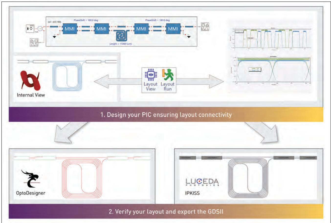
purpose photonic, electrical and optoelectronic device models, together with advanced circuit optimization and yield analysis capabilities. The VPItoolkit PDK LIGENTEC library extension adds foundry-certified simulation compact models for the standard building blocks supported by the AN800 process and enables a layout-aware schematic-driven PIC design workflow, including chip layout optimization according to the device's required optical functionality.
